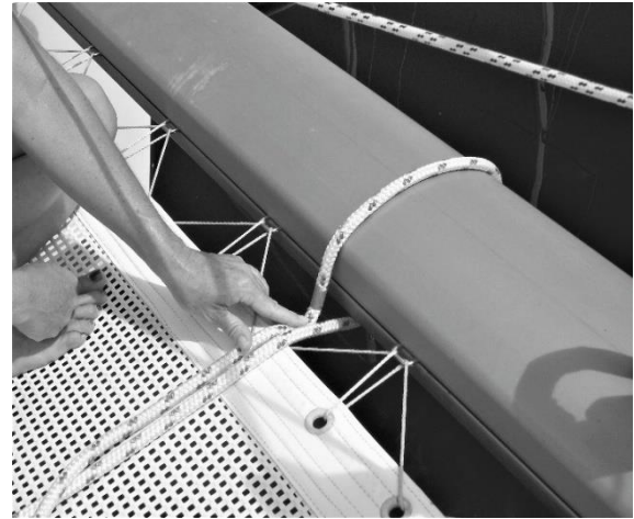
Figure 4: End of rope looped around crossbeam with point marked on rope with tape.
