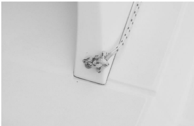
Figure 2.0: End of rope looped through a folding pad-eye.
